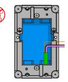
2 This step is not required, however you may connect the supplied ground wire lead to the ground wire in the wall box. If you do, then, using the supplied hardware, fasten the ground wire lead to whichever side of the mounting plate that leaves the most space for the lighting device.
